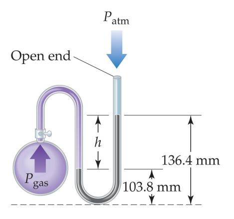
The manometer is used to measure the difference in pressure between atmospheric pressure and that of a gas in a vessel.
